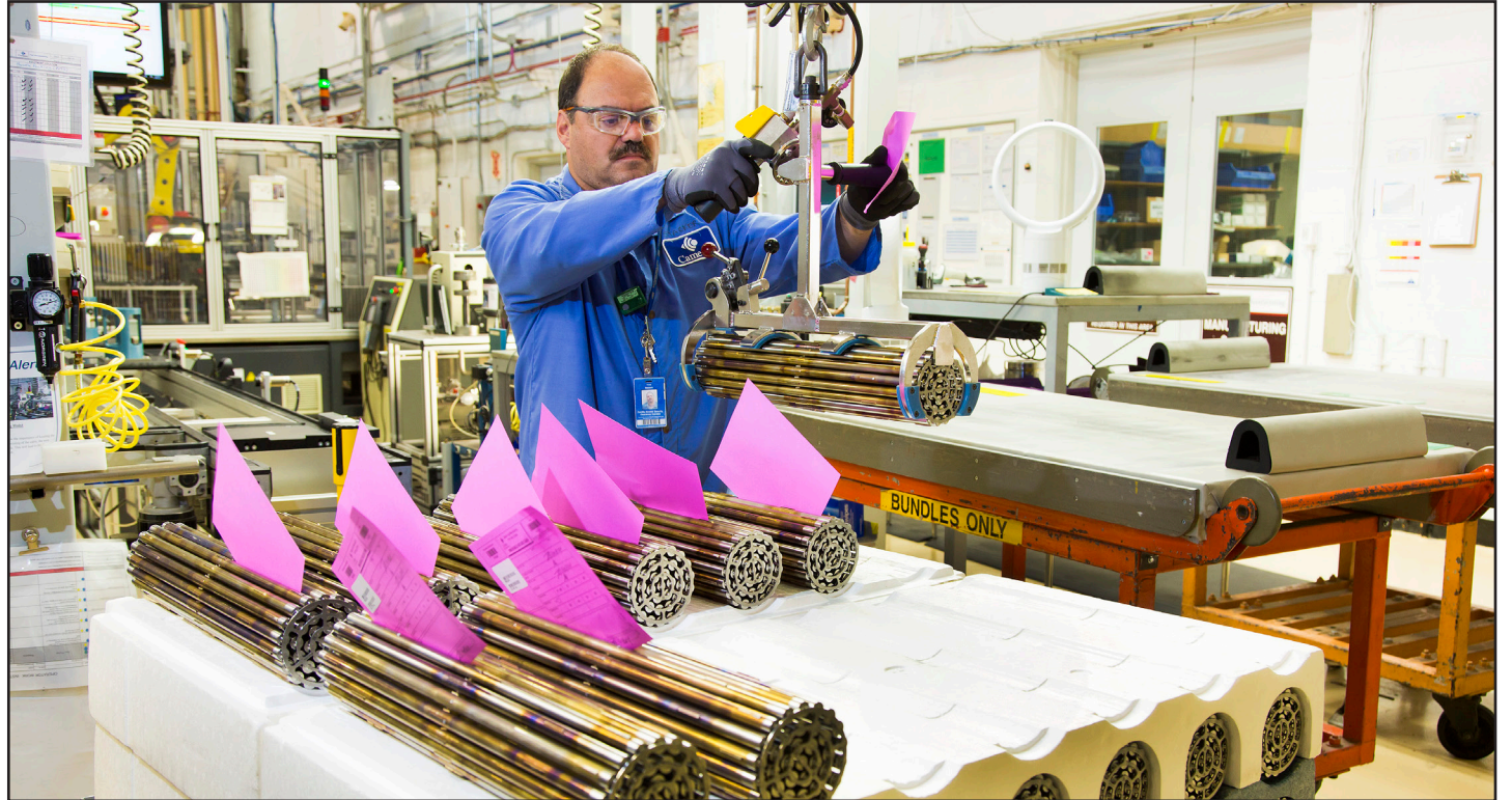
An employee packs finished CANDU fuel bundles at Cameco Fuel Manufacturing Port Hope.
